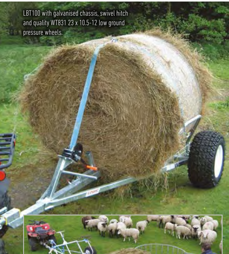
1 Back up to the bale and secure strap.
