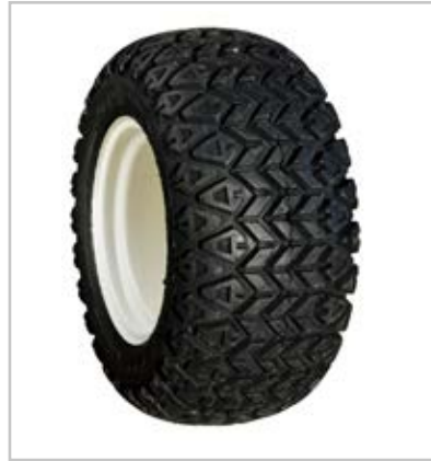
WT831 23 x 10.5 - 12 ultra-low ground pressure quality tyre for heavy duty use.
