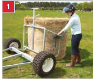
1 Back up to the bale and secure strap.
