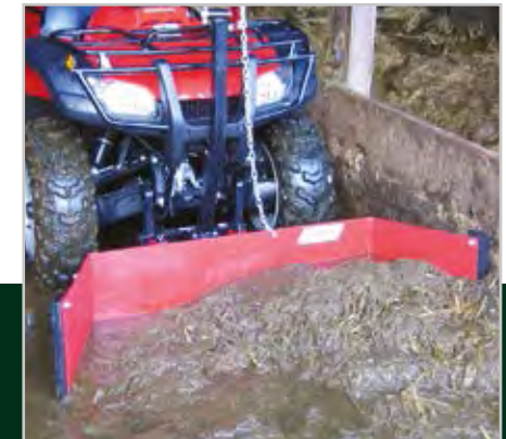
S210 yard scraper - suitable for cow sheds, cubicle houses, pig units, poultry houses, etc. With a working width of 1.3 metres, the heavy duty one piece blade is fitted with replaceable bottom and wing rubber wearing strips. Manual lift or electric ram options.
