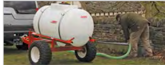
SLB600 is suitable for larger towing vehicles and features gravity discharge, with 23 x 10.5 - 12 wheels and tyres.
