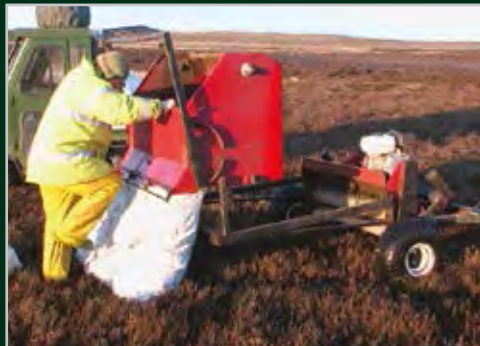
Tipping the 600 litre hopper (left) to bag off heather seed from 3 chutes ready for further cleaning and drying.
