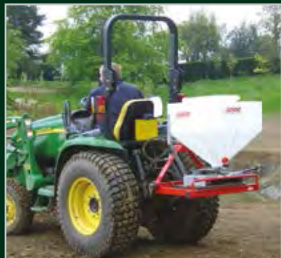
TPL115 Mounting frame (left) for 3 point linkage on tractors, suitable for larger electro broadcasters when spreading grass seed mixtures, fertilisers, etc.
