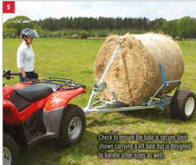
1 Back up to the bale and secure strap.
