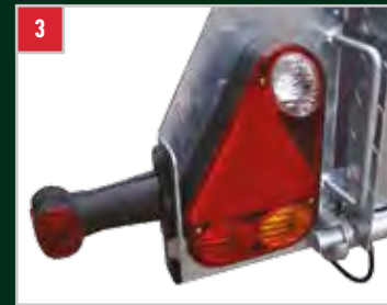
Protected light cluster with inbuilt triangle, lenses and marker lights.
