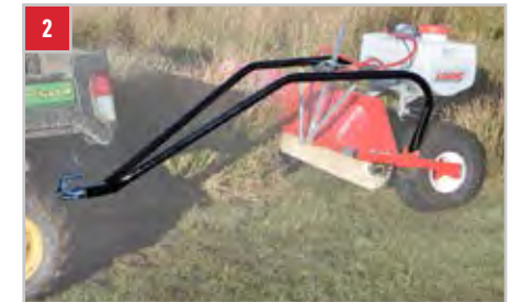
The robust 'swan neck' drawbar reduces drag in dense foliage. It can be easily moved to provide an offset facility and houses the large, in-line filter.
