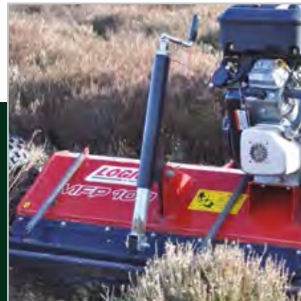
The adjustment of cutting height is controlled by a spring assisted screw jack giving cutting heights between 0-140mm on standard wheels and up to 216mm on flotation wheels.
